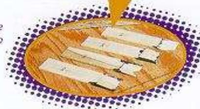
Figure 13: Wood products made from phenol-formaldehyde resins derived from bio-oil at NREL, USA
